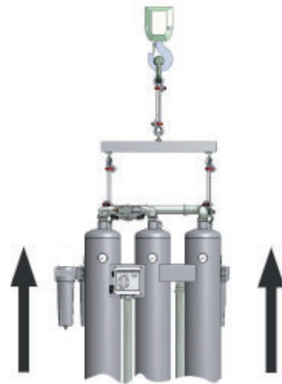
II: Installing by crane
